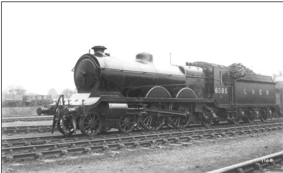
LNER class C4 4-4-2 no. 6085 at Neasden on 9 Oct. 1937. Built in 1905 it became one of the last of Robinson's Atlantics to be withdrawn in Nov. 1950 as no. 2909. photo © Railway Photographs
