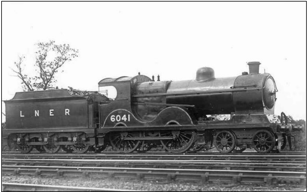
LNER class D9 4-4-0 no. 6041. This was an early design by Robinson, the first of the class appearing in 1901. They were put to work on the Marylebone expresses, displacing the less powerful class 11A 4-4-0s of Pollitt design. A superheater was added in 1913 and the Ross 'pop' safety valves were added by the LNER. No. 6041 entered BR stock as 62325 but only survived until 1950 after spending its final years shedded at Trafford Park.
