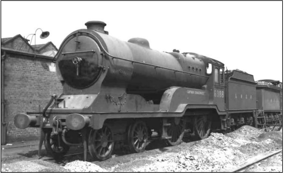
LNER class D11/2 4-4-0 no. 6388 Captain Craigenfelt at Eastfield on 31 Aug. 1938. These 'Scottish Directors' were built by the LNER to the Scottish loading gauge (lower chimney and dome) in 1924 so they were not GCR engines. They were named after characters in Sir Walter Scott's novels, following the tradition of Reid's NBR 'Scott' class (LNER class D30). The names were painted along the straight splasher. photo : L. Hanson
